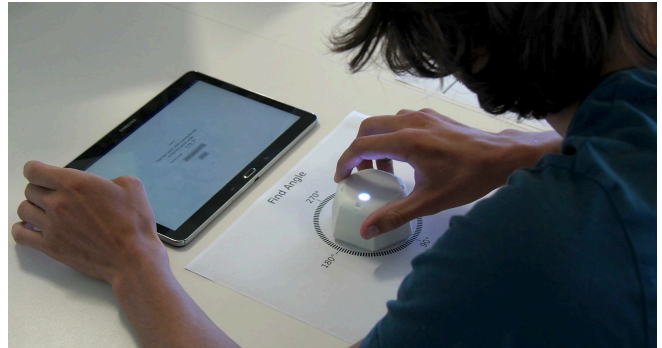
Figure 1. The Cellulo robot, conveying an otherwise hidden orientation by means of haptic feedback. By designing and assessing such “atoms” of haptic user interaction, we aim to show the usability of our robot as a haptic device and extract perceptive and manipulative measures for designing haptic elements for our learning activities.
